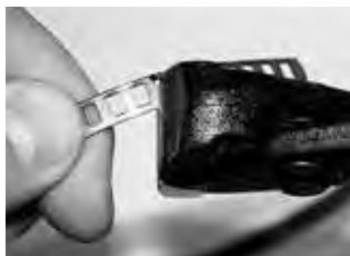
Step 3 Cut off the remaining material. To avoid possible injury deburr cut edges with a file.
